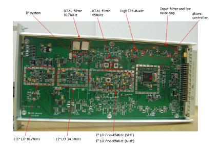
A further input (TX Test input), common for both receivers (main and diversity) is available, for the receiver self-test and for modulator calibration. Through a DSP command, the receiver can switch its input onto test signal generated inside transmission synthesizer module. That signal, amplitude calibrated by Factory, is modulated at receiving frequency and received by DSP. A fundamental test loop is close by this way.
